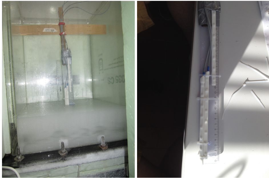
(a) Tank with the ice layer at the bottom and the frame holding the ruler and the temperature sensors. (b) The three temperature sensors sticks. The two lowermost are arranged in order to have a sensor every 1 cm, while the uppermost one has a sensor every 2 cm.
